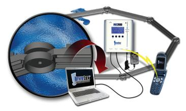
The **Aquapede** is a modular floor water sensor, created to be snapped together to form large areas of monitoring on the floor or other flat surface. It is made of a very durable plastic that is fitted with two floating metal "blades" that run parallel to one another under a durable plastic cover. This floating feature allows the blades to adjust to uneven floors and still maintain its full sensing capabilities.
