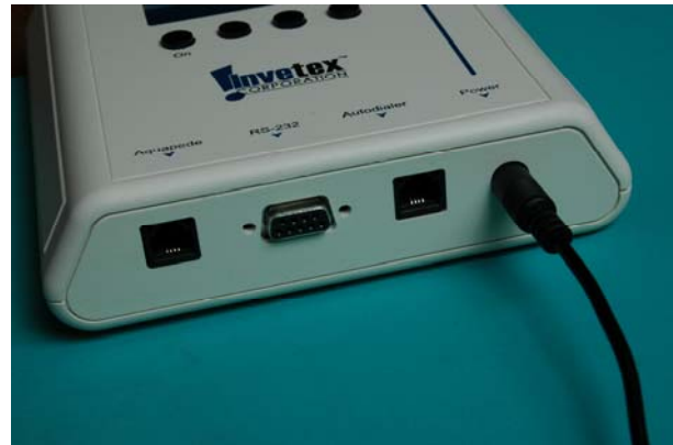
The power supply plugs into the Master Controller Box bottom.
